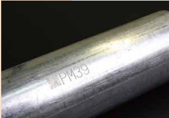
Mark 2D code on pipe.
