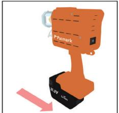
For battery installation, slide the battery all the way in until it makes a clicking sound.
