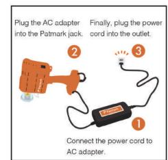
Follow the proper connection sequence. Not following the correct sequence could create a static charge in the DC output plug of the AC adapter, potentially resulting in an electric shock or minor injury. Also, make sure the adapter's plug does not touch metal parts other than the Patmark power connector.
