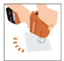
As shown in the figure, make sure to hold Patmark using both hands. Then, click the Start/Stop trigger button once and let go of the button. During the marking process, tightly hold onto the Patmark with both hands.
