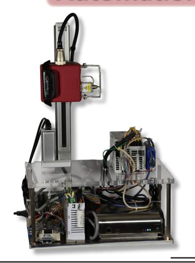
Photo to the left shows a typical automation set-up using PLC with D.I/O.
